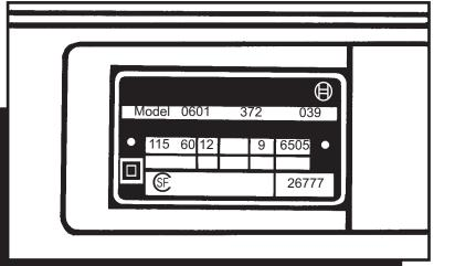
be grounded if supplied through an isolating transformer with an ungrounded secondary of not over 50 volts. Listed or labeled portable tools and appliances protected by a system of double insulation, or its equivalent, need not be grounded. If such a system is employed, the equipment shall be distinctively marked to indicate that the tool or appliance utilizes a system of double insulation.
