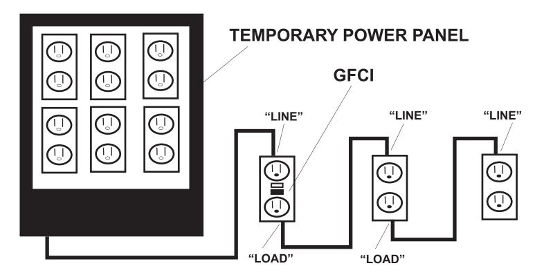
Ground fault circuit interrupters (GFCI's) are used to protect employees from electrical shocks. However, if branch outlets are not installed correctly, they will not shut off power when needed thus providing a false sense of security. Incorrectly installed GFCI's expose all contractors at the job site to potential injury as well as possible OSHA citations and fines if a compliance officer discovers the hazard.
