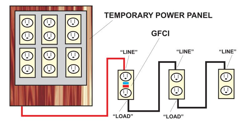
Ground fault circuit interrupters (GFCI's) are used to protect employees from electrical shocks. However, if branch outlets are not installed correctly, they will not shut off power when needed thus providing a false sense of security. Incorrectly installed GFCI's expose all contractors at the job site to potential injury as well as possible OSHA citations and fines if a compliance officer discovers the hazard.
