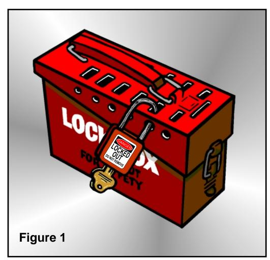
figure 1. It is most used during shutdowns. The main power panel is locked out with one lock, and the key is placed in the lockbox. supervisor of the operation puts his own personal lock on the front of the lockbox, and the rest of the personnel involved put their personal locks on the side holes, keeping the lid closed. The main power panel key cannot be retrieved until all personnel have removed their locks.
